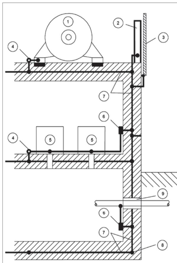
Interconnected concrete encased steel will work as a “Faraday Cage” and limit the EMP effects of a nearby and distant lightning strike too. Equipotential bonding of different steel installations and steel reinforcement in a building not only reduce the failure of electronic equipment, but increase the life of equipment too. This method of Equipotentialisation (Protective Bonding) is well accepted and appreciated by the structural engineers.
